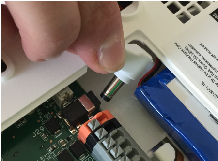
Plug in the power connector
