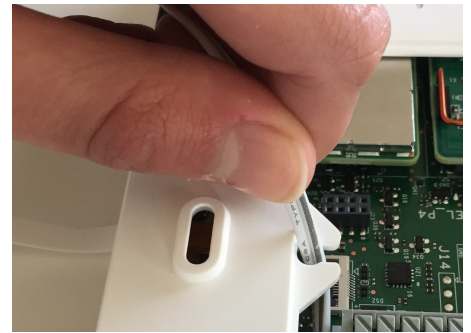
Insert the wire into the strain-relief
