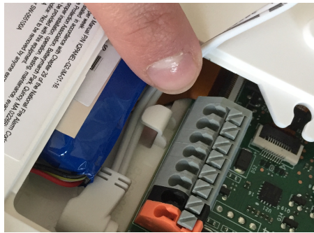
Route the wire behind the retainer clip
